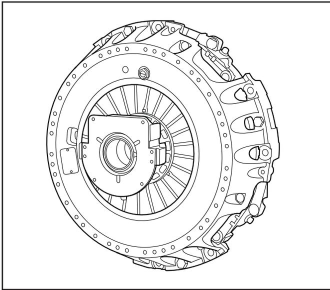
*Twin XTend automatically adjusts for clutch wear; no manual adjustments required.*
