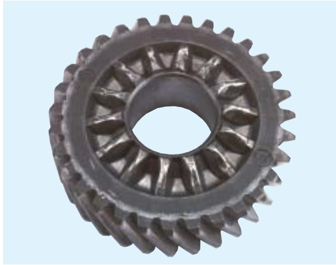
Helical Side Gear - Bushing Burn-Up
