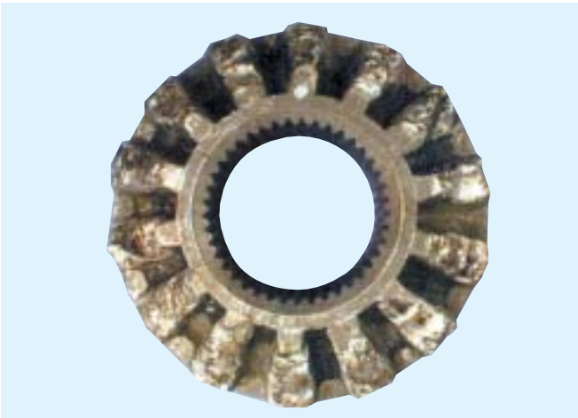
Side Gear - Catastrophic Shock
