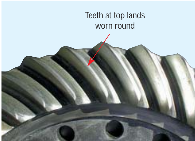
Ring Gear - Low Lube - Crows Foot
