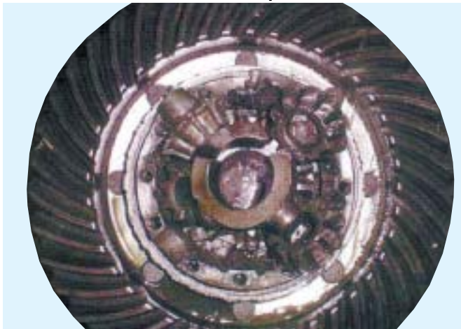
Wheel Differential - Catastrophic
