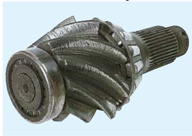
Drive Pinion - Low Lube - Scoring
