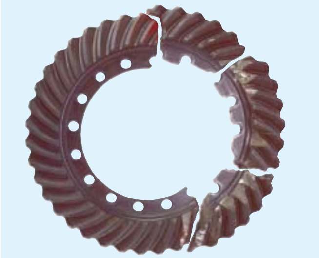
Drive Pinion - Torsional Shock Failure
