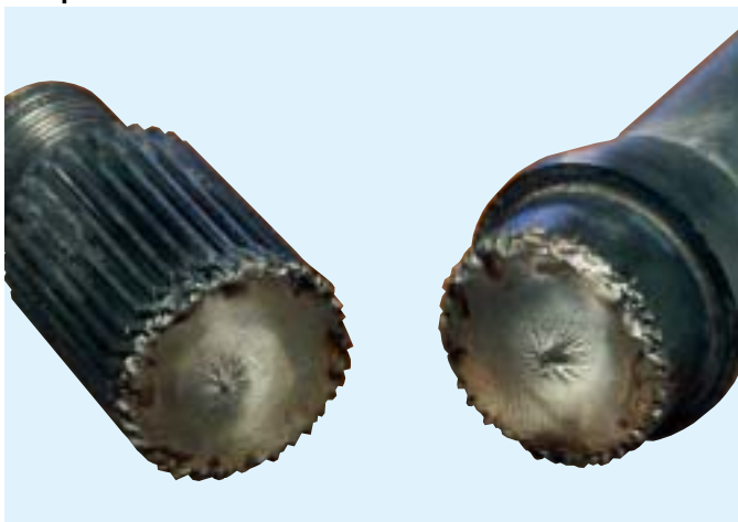
Output Shaft - Torsional Shock Failure
