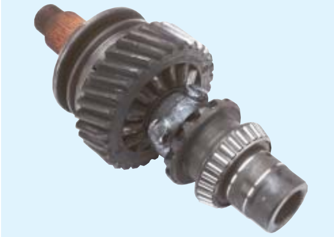
Helical Side Gear - Bushing Burn-Up
