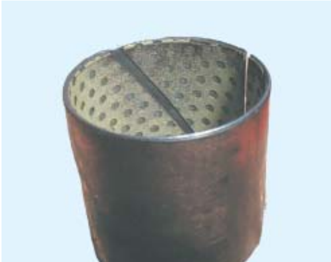
Bushing Worn in One Area Only
