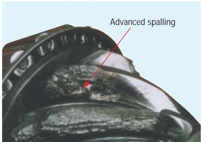
Drive Pinion - Spalling
