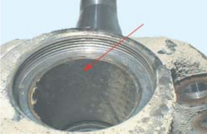
Bushing - Lack of Grease
