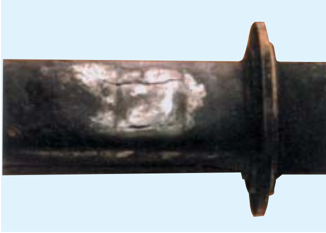
Loose Clamping Hardware
