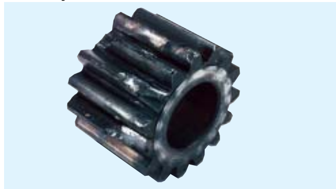
Planetary Gear - Shock Failure
