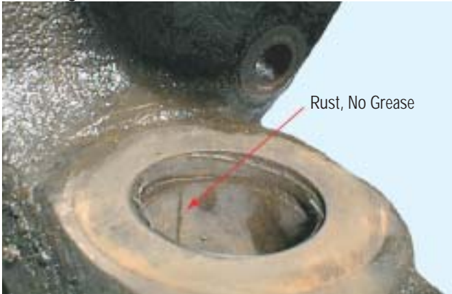
Bushing - Lack of Grease
