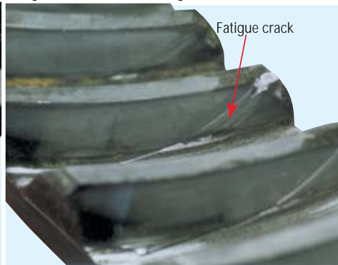
Drive Pinion - Tooth Fatigue Failure
