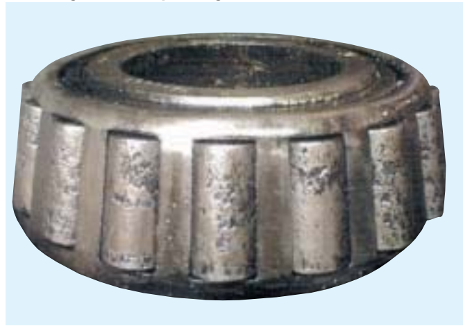
Bearing Cone - Spalling
