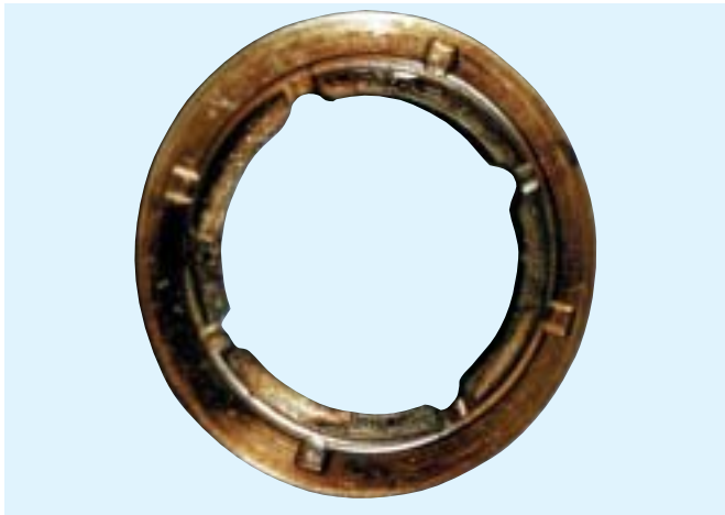
Power Divider Thrust Washer - Lubricant Contamination
