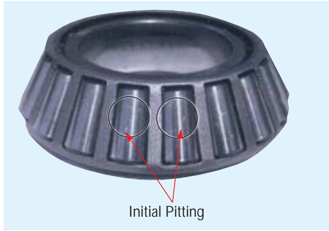
Bearing Cone - Spalling
