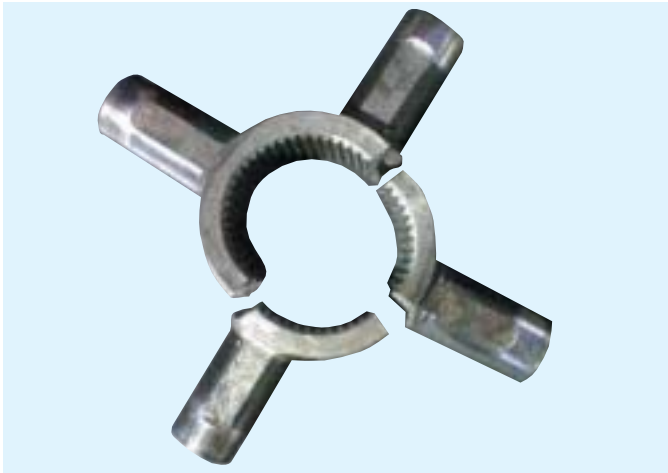
Sliding Clutch - Shock Failure
