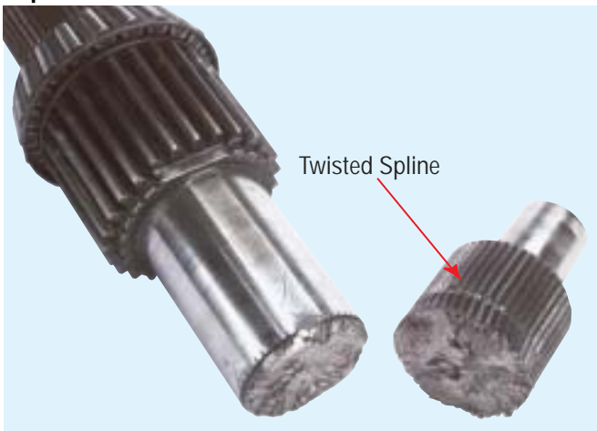
Input Shaft - Torsional Shock Failure
