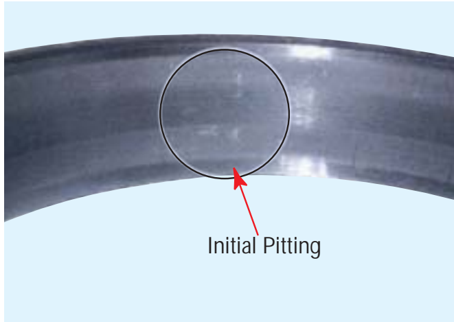
Bearing Cup - Spalling
