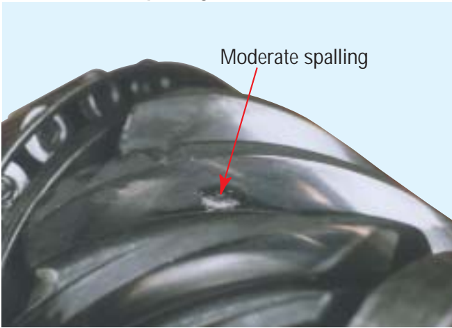
Drive Pinion - Spalling
