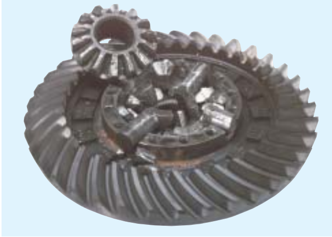
Side Gear - Catastrophic Shock
