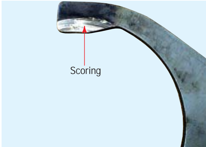
Power Divider Thrust Washer - Lubricant Contamination
