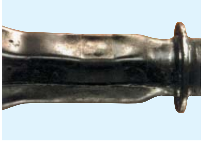
Over-torqued Clamping Hardware
