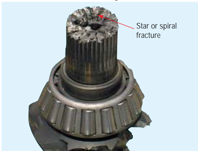
Drive Pinion - Torsional Fatigue Failure
