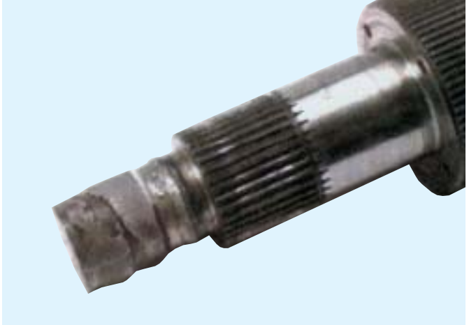
Output Side Gear - Stub-End Bore Galling
