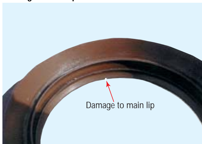
Damaged Seal Lip
