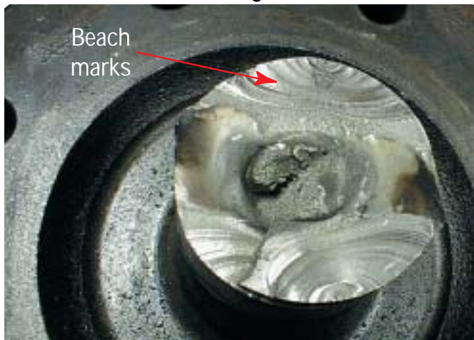
Axle Shaft - Torsional Fatigue Failure
