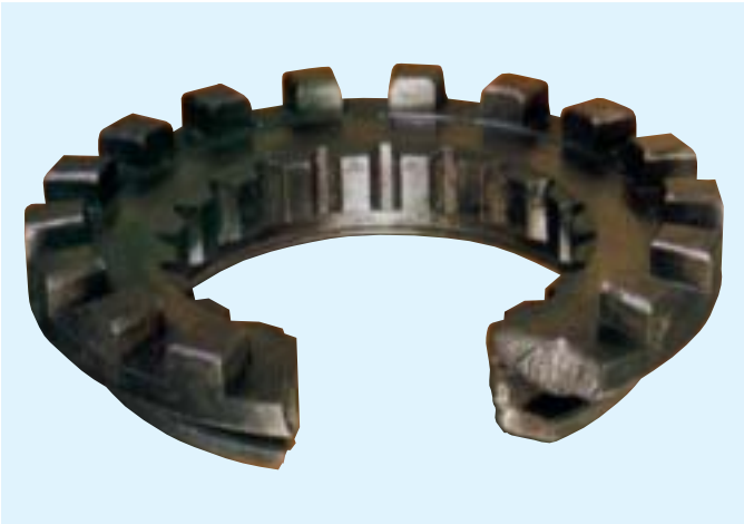
Sliding Clutch - Shock Failure
