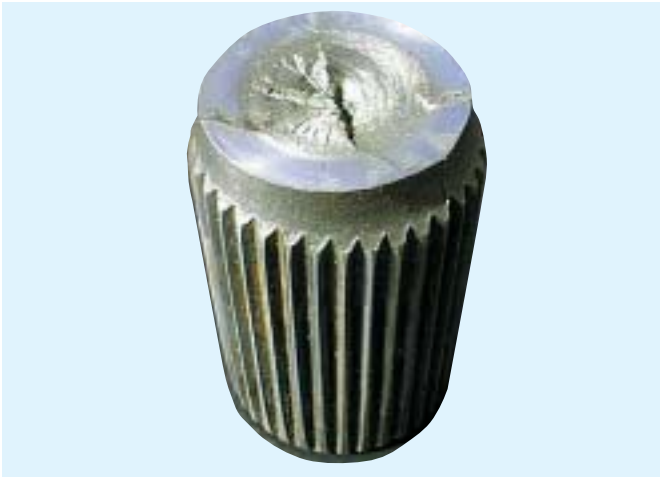
Axle Shaft - Torsional Fatigue Failure
