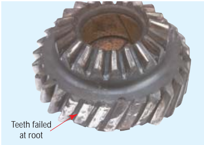
Input Shaft - Torsional Shock Failure
