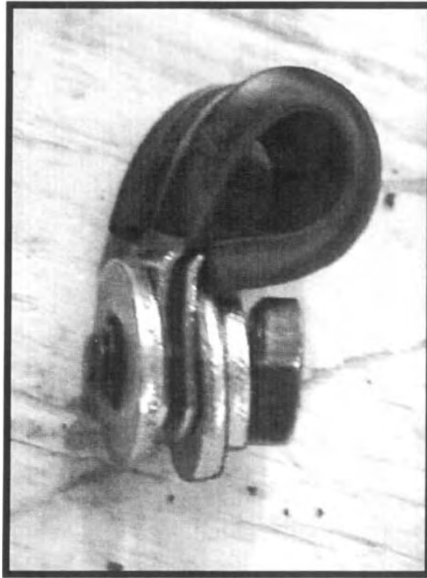
Figure 10.2: Clamp Assembly, ABS Cable, Inside Steerable End
