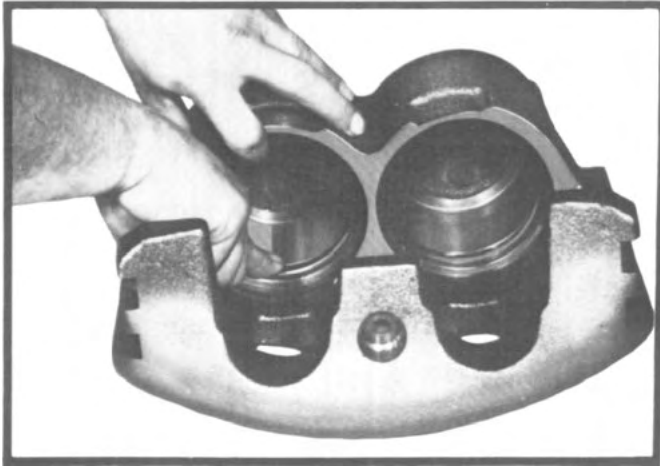
Fig. 31 — Installing piston seal in caliper groove.
